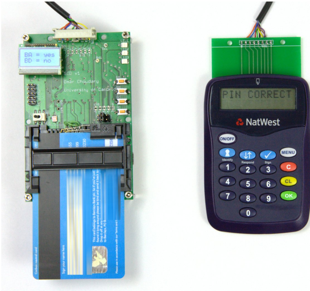
Figure 6.2: Forward Commands application tested on Natwest CAP reader. The SCD has blocked the transaction after the PIN has been entered and is waiting for the user to select if the transaction should continue (yes) or not (no)
