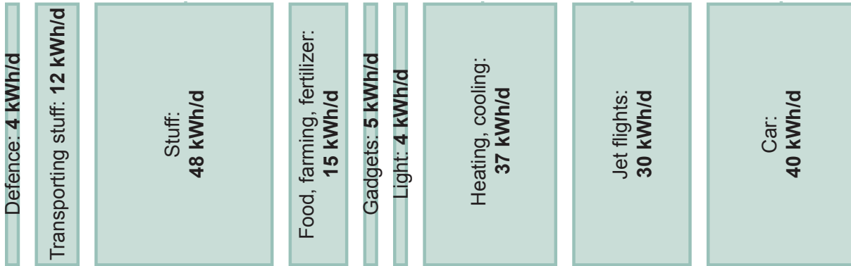
Figure 3.1: Estimated energy consumption of a “typical moderately-affluent person”
